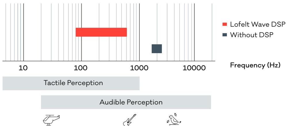
An example of audio events at 2000 Hz being processed into the key haptic sensitivity frequency range.
