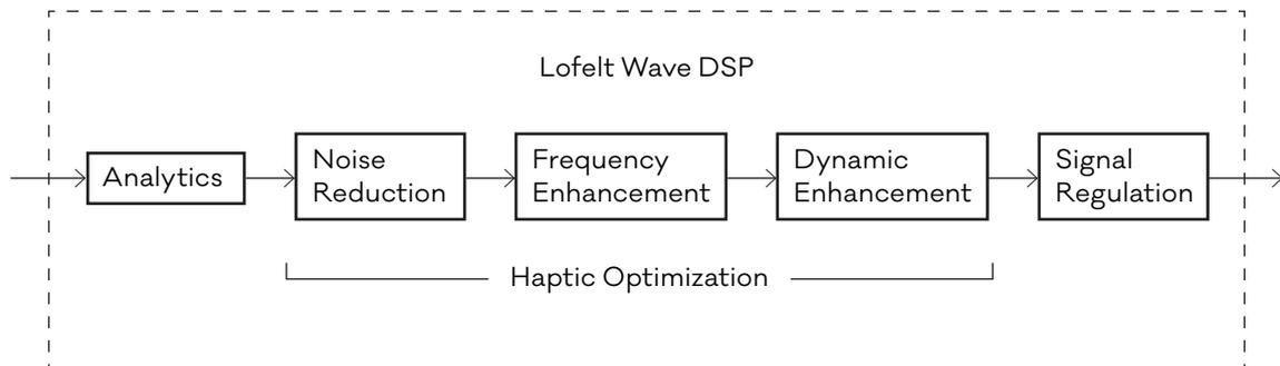
*Lofelt Wave DSP incorporates analytics, noise reduction, frequency enhancement, dynamics enhancement and signal regulation components for real-time signal flow optimization.*
