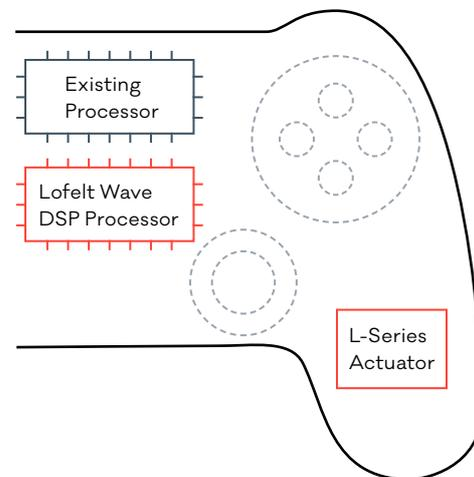
*Lofelt Wave DSP can run on the hardware platform’s existing processor or a standalone processor.*
